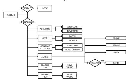
Figure 3.7 Flow Chart for Alarm 2
